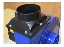
Place the outlet hose adaptor over the gasket and fix it to the flange using 6 M6 x 20mm hex head bolts, washers and nuts.
