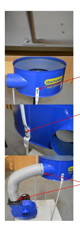
Bolt on the three collector support arms, making sure that the tops are cranked inwards.
