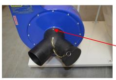
The fan inlet is 125mm diameter. It can be used directly with a 125mm diameter hose. For most applications it is preferable to use 100mm diameter hose.
