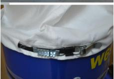
Feed the plain end of the second flexible clamp through the slit at the bottom of the filter bag and keep pushing until it emerges from the other slit. Clamp it, as shown and your extractor is ready for use.
