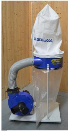
Fit the transparent plastic bag over the bottom of the collector and secure it with one of the flexible clamps.
